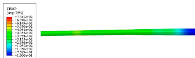
Figure 8. Barrel temperature field under 90 rounds of continuous shooting.
