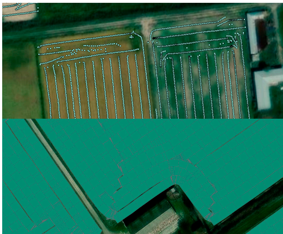
Figure 2. Different vector data types of yield recordings after insertion into the study's GIS; upper side: point data type; bottom side: polygon data type.
