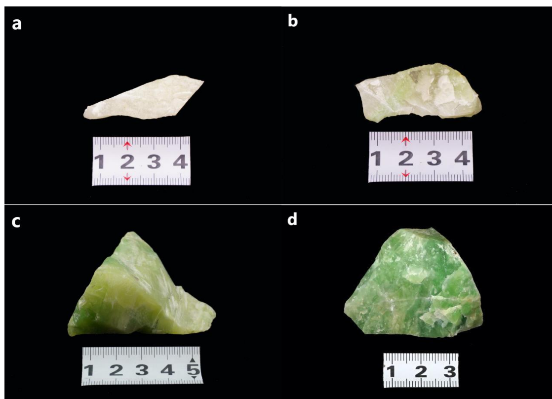
Figure 1. Sample photographs. (a) ZB-3: White patches within a white matrix. (b) ZB-2: Fibrous green inclusions embedded in a white matrix. (c) ZB-1: Yellowish-green matrix containing white veinlets, emerald-green spots, and fibrous green inclusions. (d) ZB-4: Light green matrix exhibiting dark green patches, fibrous green inclusions, and white veinlets.
