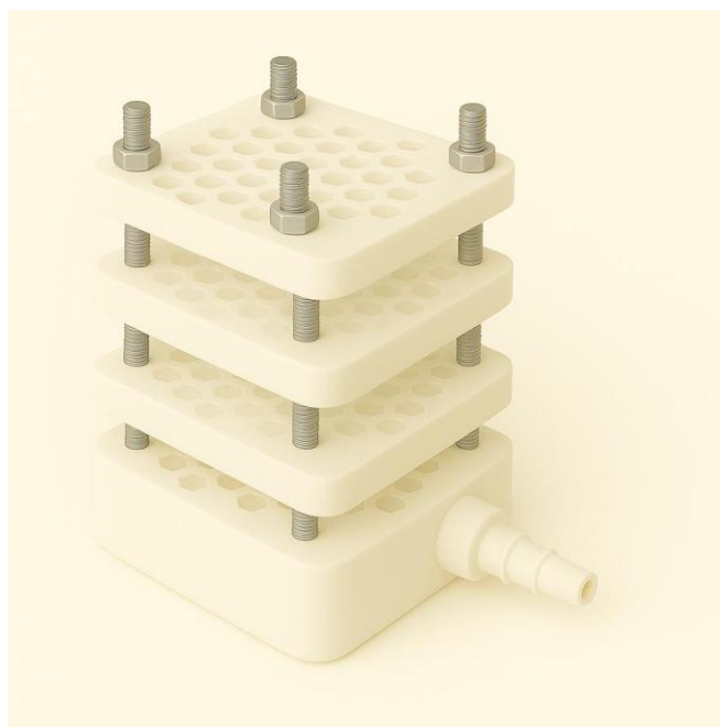
Figure 1. Illustrative exploded schematic of the NP-TRAP device highlighting its main conceptual components. The top layer allows passive influx of nutrients and substrate-derived molecules from the environment and remains unsealed by membrane. The second layer contains 56 hexagonal cultivation chambers arranged in a honeycomb pattern and is separated from the top layer by a 0.2\ \mu\text{m} microfiltration (cell-excluding) membrane, enabling molecular diffusion while excluding cells. The third layer, designed for metabolite capture, is also separated by a 0.2\ \mu\text{m} microfiltration membrane and houses adsorbent resins or compound-selective membranes. A unidirectional diaphragm layer with duckbill-type silicone check-valves, beneath an additional 0.2\ \mu\text{m} microfiltration membrane, prevents reflux. All layers are aligned through peripheral orifices and secured using stainless steel rods and nuts. The bottom cap includes a lateral vacuum outlet fitted with a non-return valve for mild suction.
