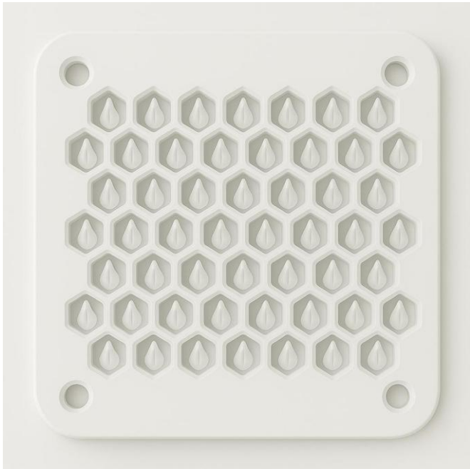
Figure 3. Diaphragm interface integrated into the top of the bottom cap. Each hexagonal compartment is fitted with a central duckbill-type silicone valve to ensure unidirectional flow and prevent backflow or cross-contamination. This configuration enables passive or suggested mild vacuum-assisted metabolite transport from the cultivation chambers into the capture layer.
