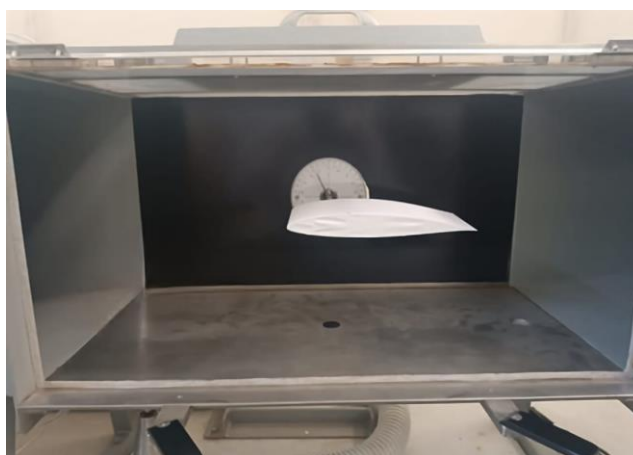
Figure 8. Experimental setup for subsonic wind tunnel testing.
