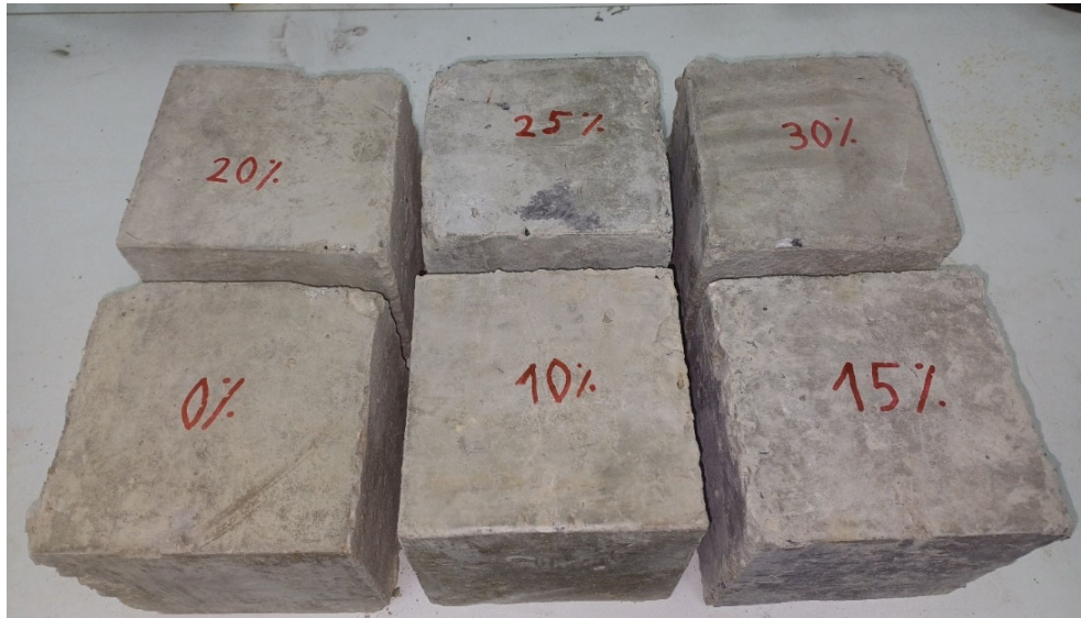
Figure 12. Concrete cubes from each mixture with different e-waste percentages.
