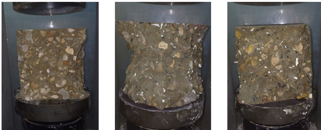
Figure 11. Concrete cubes compressive test failure with increasing e-waste percentages.
