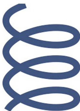
Figure 2. Shown is the helix of radius R and pitch h generated by constant curvature and constant torsion as in Eq.(10) below. R is the radius of the helical cylinder and for every 2\pi rotation around the cylinder axis the curve rises a height h .
