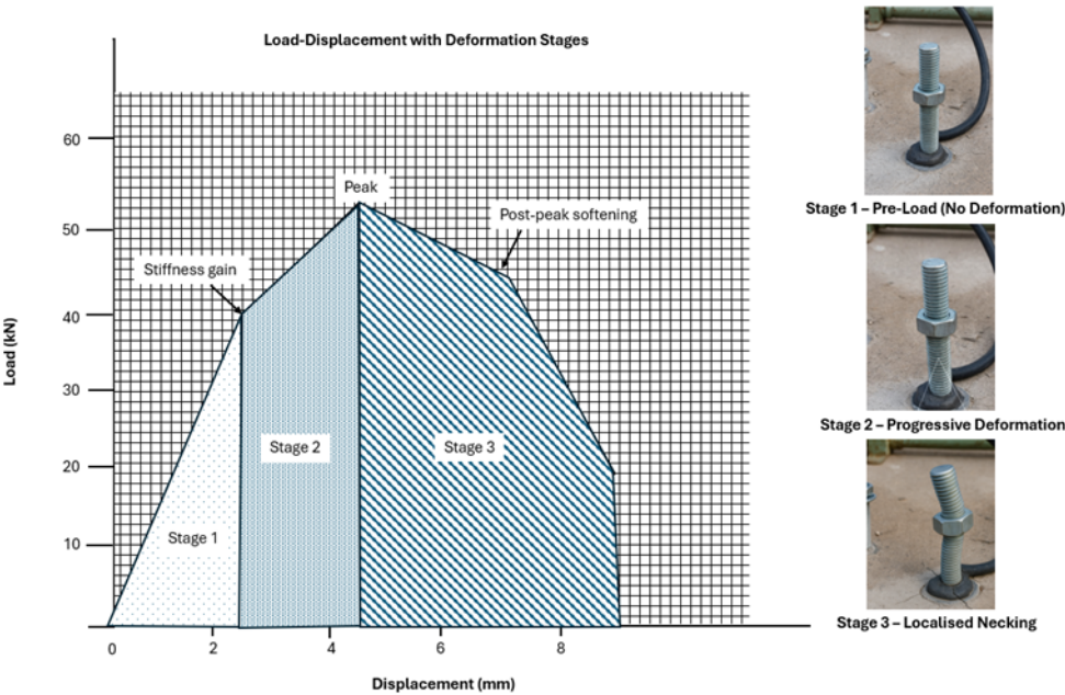
Figure 12. Load–displacement response of an M16 vinyl-ester bolt in intact rock, showing stiffness gain, peak capacity and post-peak softening.
