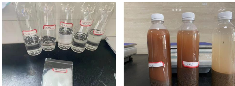
Figure A2. Left image: A PAM flocculant powder specimen used in this study and aqueous solutions of the PAM flocculant with different concentrations; Right image: Commercially manufactured sand soaked in pure water, 0.006% and 0.01% aqueous solutions of the PAM flocculant for one hour, respectively.
