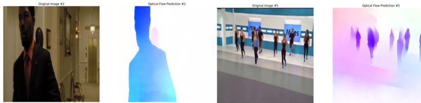
Figure 3. Sample optical flow outputs generated by the UniMatch model from XD-Violence dataset.
