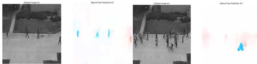
Figure 2. Sample optical flow outputs generated by the UniMatch model from UCSD Ped2 dataset.
