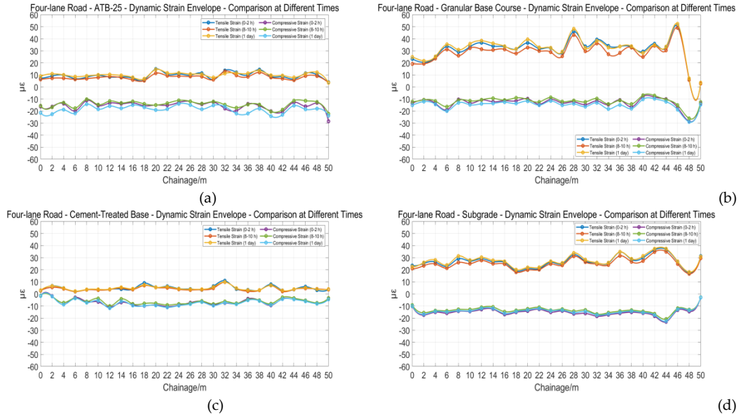
Figure 12. Time-Resolved Dynamic Strain Envelopes in Multilayered Pavement (Four-Lane Road) (a)ATB-25; (b) Granular Base Course; (c) Cement-Treated Base; (d) Subgrade.
