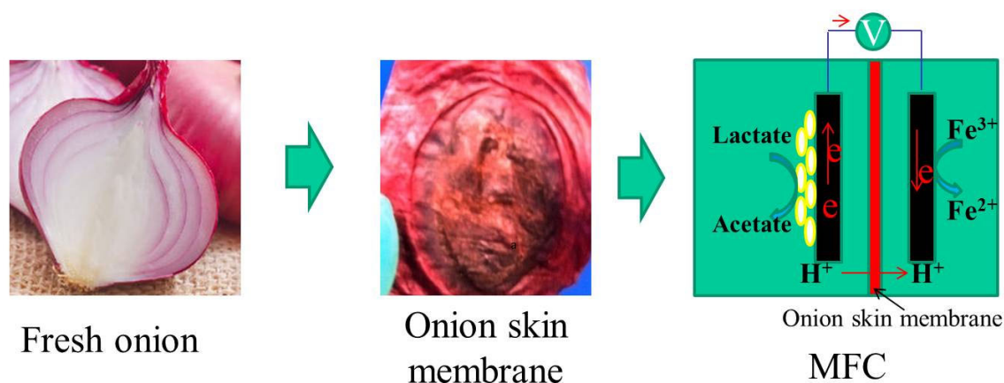
Figure 1. Photograph of onion skin, prepared onion skin membrane and the prototype of onion skin membrane equipped MFC.
