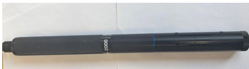
Figure 3. The AquaSond-2000 (AS-2000) multiparameter water quality monitoring sonde used for continuous monitoring during the study period.
