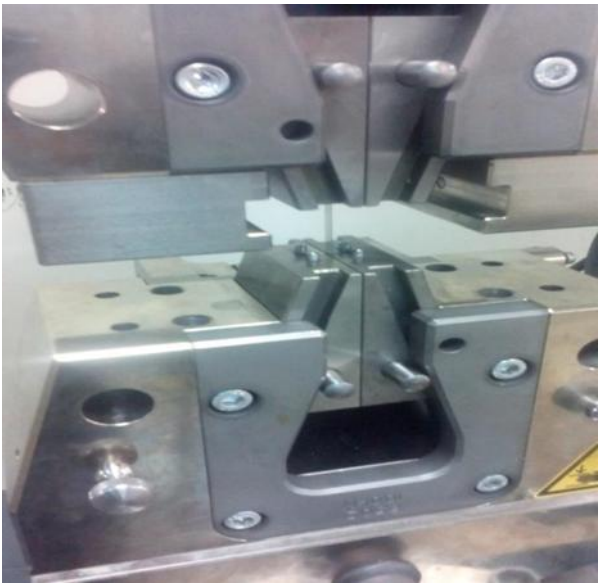
Figure 2. Mounting of tensile specimen in the testing machine.
