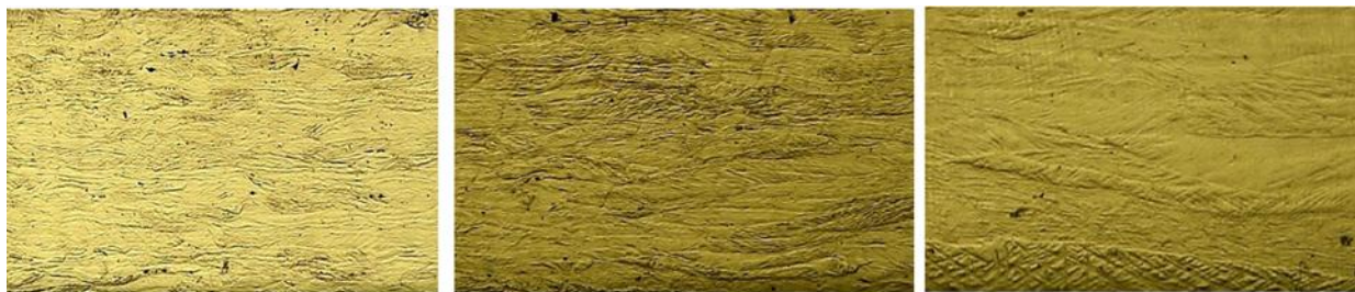
Figure 4. Optical micrographs of the cold-rolled AISI 304 sheet showing elongated austenitic.
