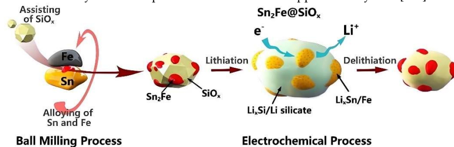
Figure 11. Illustration of preparation and electrochemical reaction for the \text{Sn}_2\text{Fe}@\text{SiO}_x composites [186].
