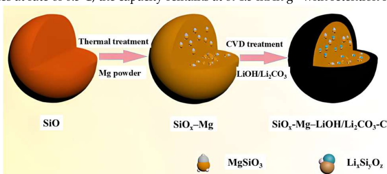
Figure 9. Schematic illustration of the synthesis process of \text{SiO}_x\text{-Mg-Li}_2\text{CO}_3/\text{LiOH-C} . [148].
