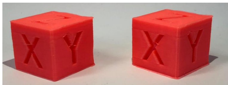
Figure 14. Calibration Cube 50mm/s (left) next to Calibration Cube 100mm/s (right).
