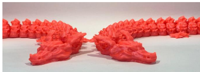
Figure 16. Articulated dragon 50mm/s (left) next to articulated dragon 100mm/s (right).
