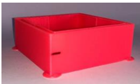
Figure 13. Pressure Advance Tower with a marking at the height with the sharpest corners.
