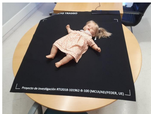
Figure 4. Prototype of the Sensing Tex pressure mat used in the study, with a mannequin illustrating the capture of the pressure imprint.
