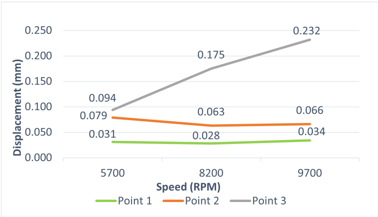
Figure 10. Graph of Displacement Levels in the Cutting System Using Chainsaw Across Various Area Points with Speed Variations.
