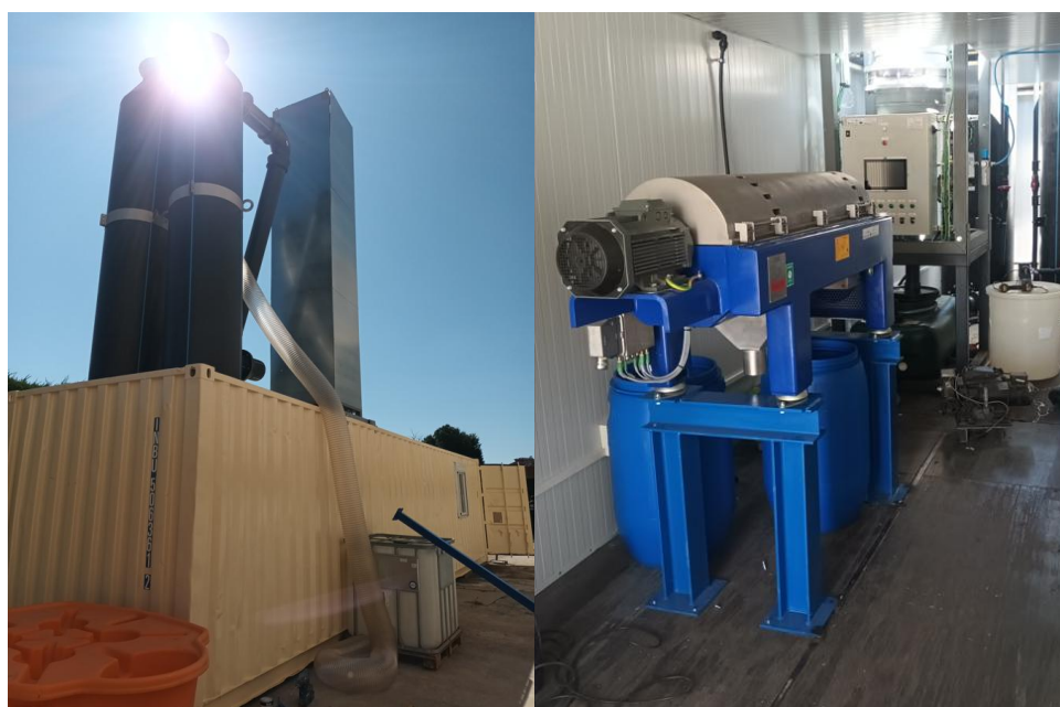
Figure 1. Pilot-scale nutrient recovery system installed at the Valladolid municipal wastewater treatment plant, combining ammonia stripping and struvite crystallization. Source: CARTIF.
