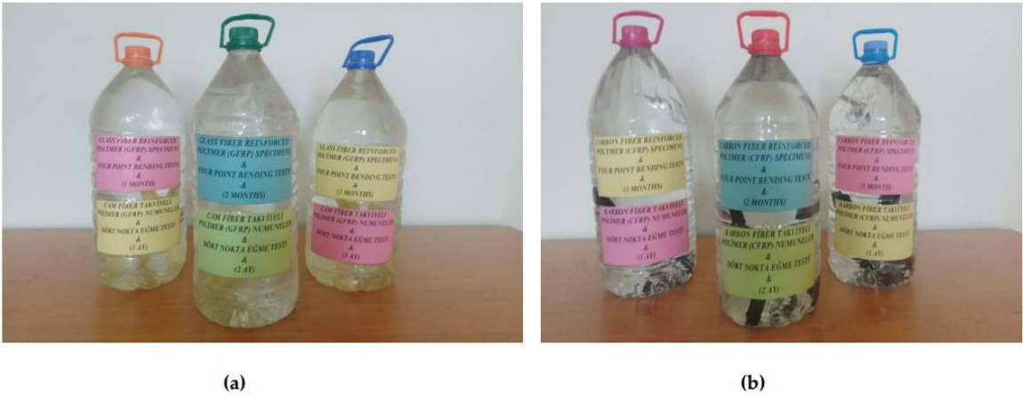
Figure 6. Soaking of GFRP (a) and CFRP (b) samples in seawater with 3.3–3.7% salinity for 1, 2 and 3 months.
