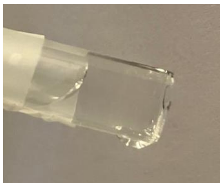
Figure 5. Double meniscus formed by water adhesion to glass tube walls.
