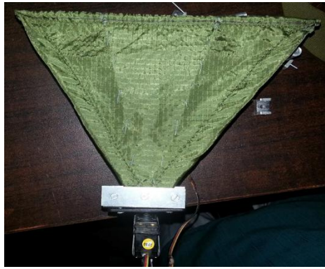
Figure 38. Tail along with servos after complete fabrication process.
