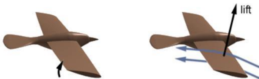
Figure 1. Twist of wings and Production of Lift and Thrust.
