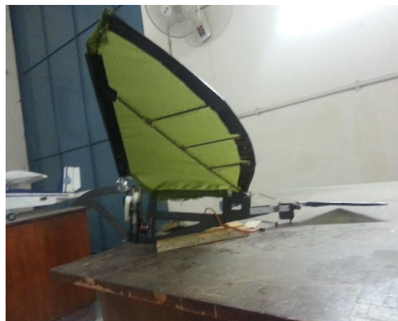
Figure 40. Side view of assembled flapping wing micro aerial vehicle.
