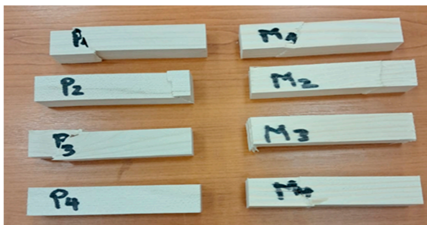
Figure 8. Fracture patterns of wood in compression parallel to the wood fibers.
