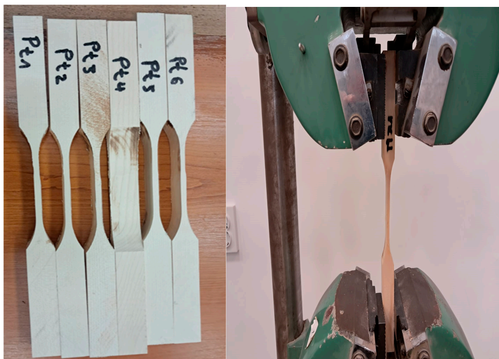
Figure 2. Determination of the tensile strength parallel to the wood fibers: a- sample shape; b-fixing in the blades of the tensile testing machine.
