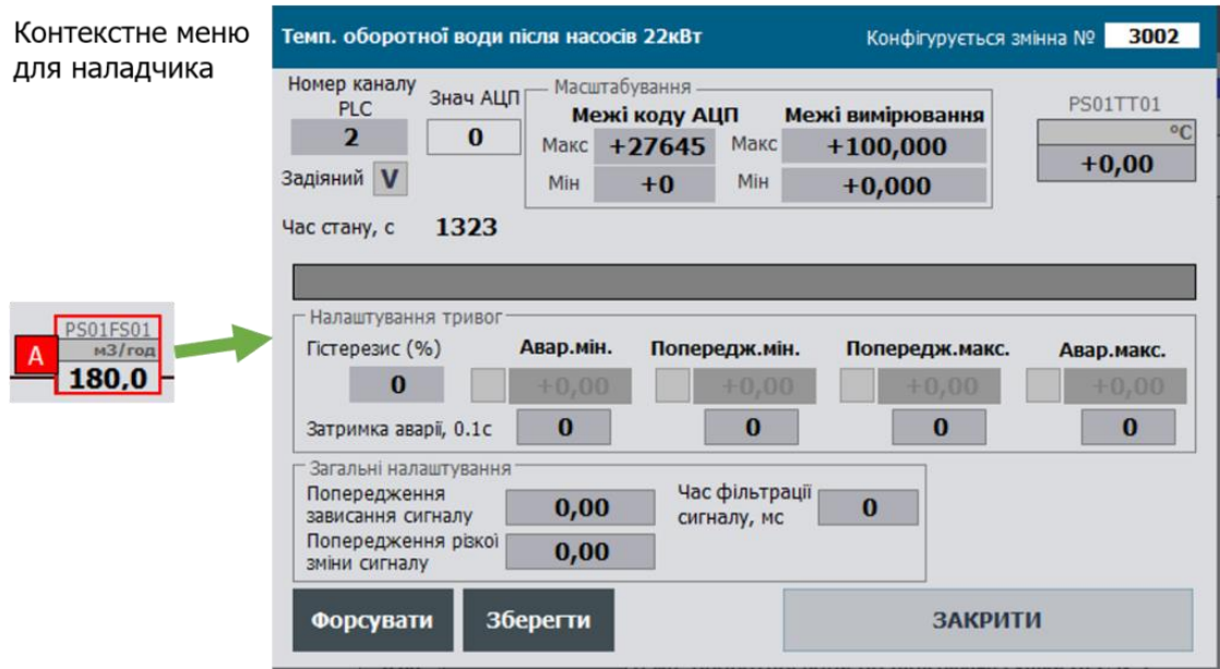
Figure 21. Example of contextual configuration: right-click triggers a pop-up configuration screen (implemented in Citect SCADA).
