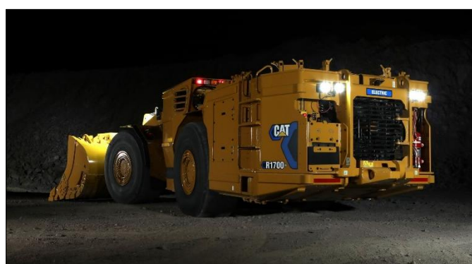
Figure 2. Battery-electric underground loader (LHD) (R1700 XE) 14.
