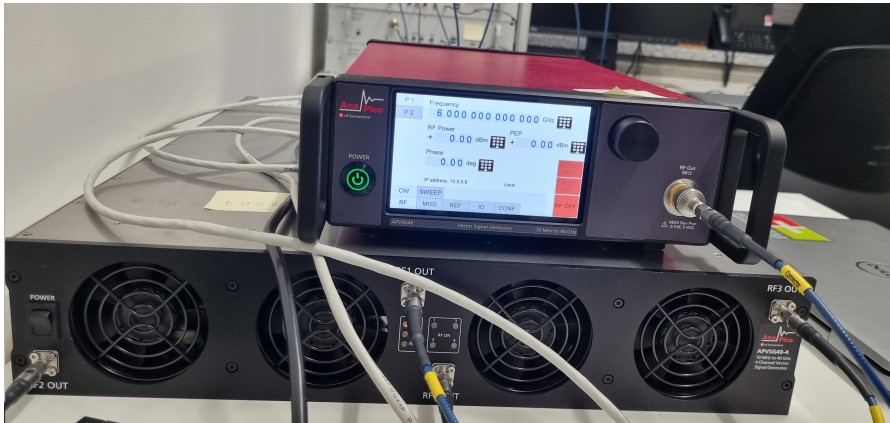
Figure 19. Close-up of the AnaPico APVSG40 stack. The red unit (top) acts as a jammer. The black unit below provides four phase-coherent data channels.
