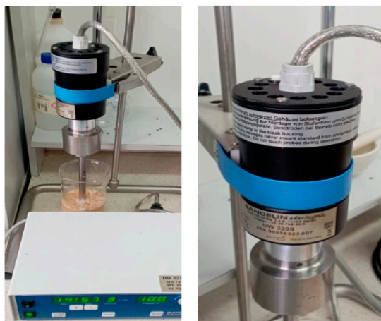
Figure 5. Ultrasonic homogenizer (BANDELIN Sonopuls HD 2200, MS 72 probe) used for UAM.
