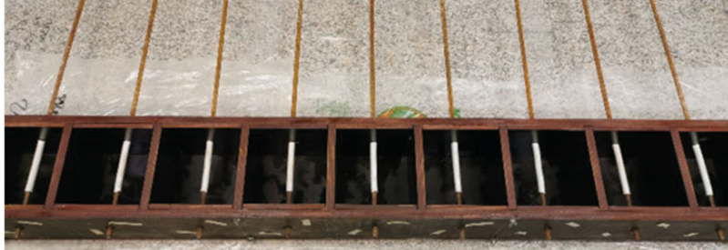
Figure 2. Special molds with integrated openings for bar placement.
