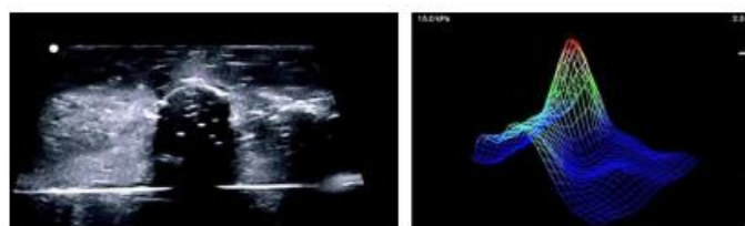
Figure 6. Ultrasound image (left) and Tactile Imaging output (right) of a breast phantom, illustrating complementary structure and biomechanical data[109].
