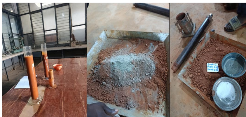
Figure 2. Hydrolysis Test, Cement and NaOH mixing & compaction.
