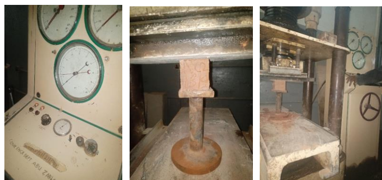
Figure 3. Compressive strength test on cubes.
