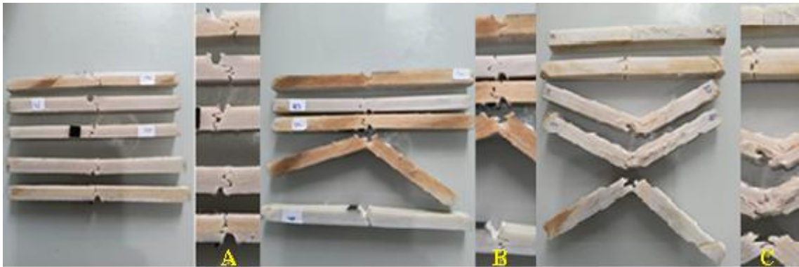
Figure 9. Some fracture profiles in intact specimens. (9A) 40%, (9B) 50% and (9C) 60% fiber theoretical volume fraction.
