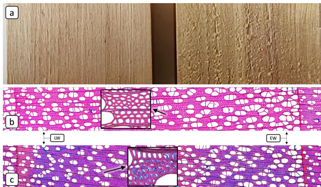
Figure 2. Overview of specimen selection. (a,b) Comparison of specimens with a smooth surface (left) and a “woolly” surface (right). The woolly surface serves as a macroscopic indicator for tension wood (TW). (b) Light microscopic image of an annual ring from an area of normal wood (NW). (c) Light microscopic image of an annual ring from an area of tension wood (TW). Safranin stains the lignin in lignified cell walls red, while astrablue stains cellulose blue. Since the distinctive G-layer of TW consists primarily of cellulose, TW areas can be identified by their blue staining, whereas NW areas appear red.
