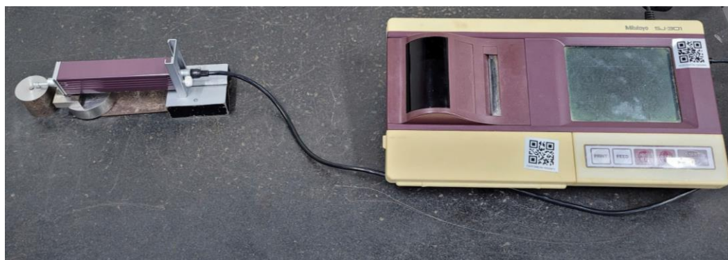
Figure 2. Surface roughness measurement using the Mitutoyo SJ301 tester.
