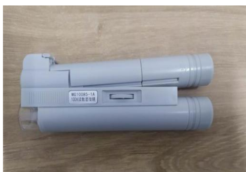
Figure 7. MG10085-1 reading microscope.
