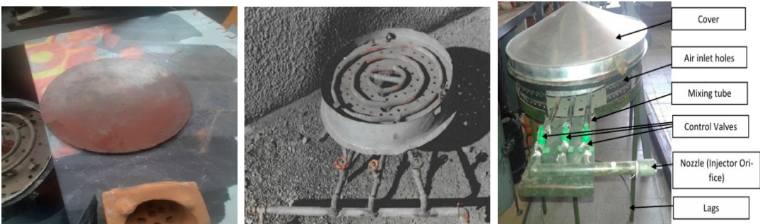
Figure 1. steel-pipe burner composed of three concentric rings[17].
