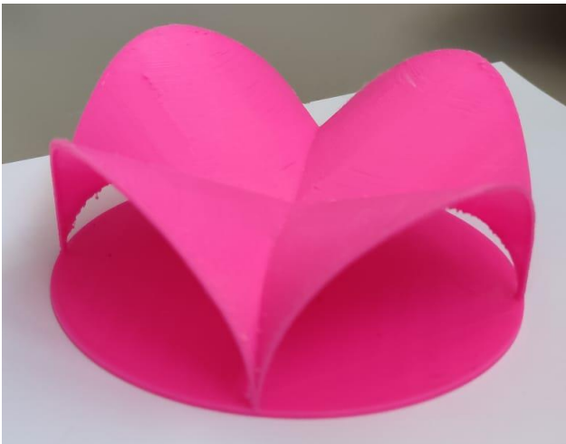
Figure 12. Scale Model of Crossing adapted to four linear connections.
