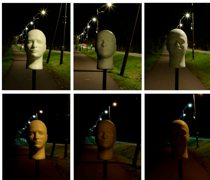
Figure 7. shows the appearance of the heads under the conventional (top) and alternative (bottom) luminaire. The photos were taken on a different day from the actual experiment, using the same shutter speed to simulate the perceived difference in brightness.
