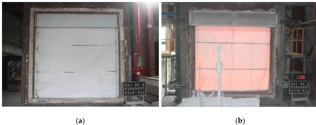
Figure 6. Fire resistance test of fire shutter using 3 m × 3 m vertical furnace: (a) before testing; (b) after testing.
