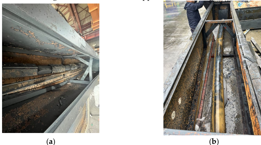
Figure 5. Deflection of barrel and barrel support bracket after fire resistance test: (a) immediately after fire resistance test; (b) after 24 hours.
