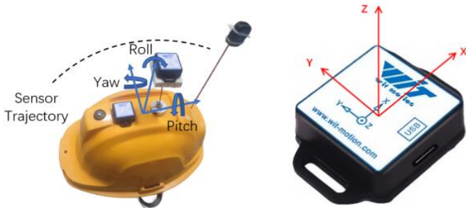
Figure 5. MEMS Attitude Sensor Layout and Sensor Coordinate System
