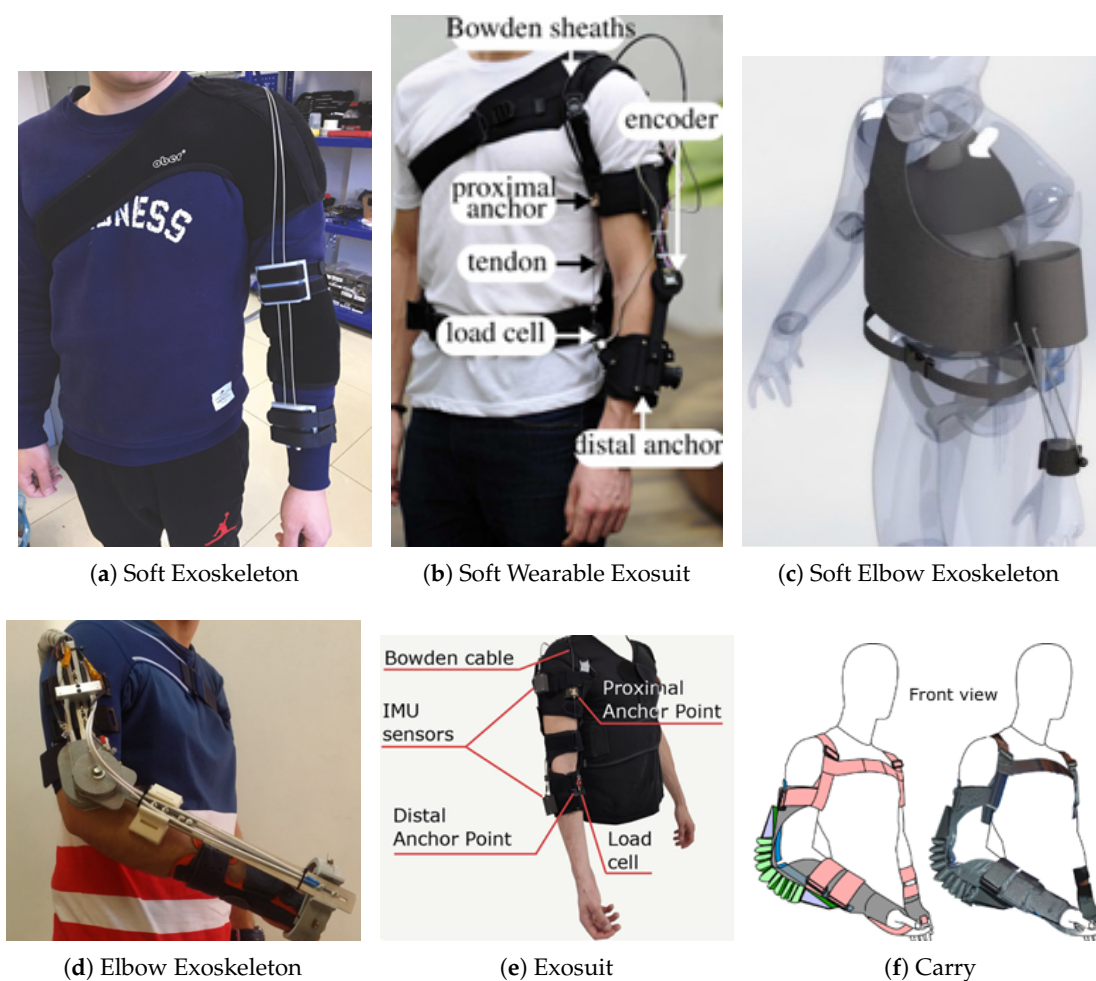
Figure 3. Prototypes of the elbow exoskeletons. (a) Soft exoskeleton actuated by a cable-driven mechanism (Bowden cable), incorporating a force sensor for feedback control [23]. (b) The soft wearable exosuit utilizing a cable-driven actuator (Bowden cable), also integrated with a force sensor for motion assistance [24]. (c) A Soft elbow exoskeleton employing a motor tendon actuator, equipped with an infrared sensor, capable of both flexion-extension and supination-pronation movements [25]. (d) An elbow exoskeleton actuated by shape memory alloy (SMA) wires, supporting both flexion-extension and supination-pronation [40]. (e) The Lightweight exosuit with an inertial measurement unit (IMU) sensor, actuated via Bowden cable for motion assistance [6]. (f) "Carry" a pneumatic elbow exoskeleton that uses force sensors to provide assistive support [32].
