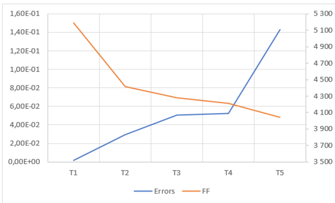
Figure 5. Graph of the tradeoff between the Resources used (FFs) and Errors of the output values (Maximum Absolute Value) when the wordlength decreases. The left axis corresponds to the Errors. The right axis corresponds to the number of FF's.
