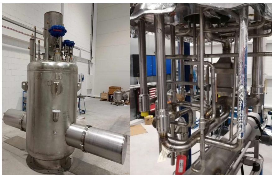
Figure 14. The vacuum vessel and interior space of the valve box.
