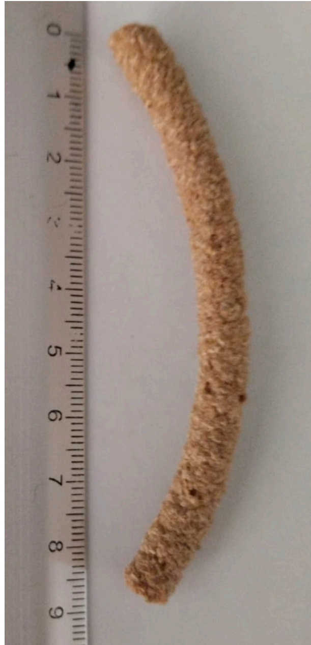
Figure 12. The final extrudate was obtained at optimal processing conditions (144 °C and 207 rpm).
