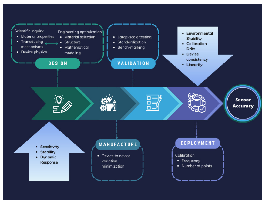
Figure 3. Step graph of an approach to sensor accuracy assurance during the design, manufacturing, validation, and deployment of a sensor technology, factors to consider are highlighted in blue in the first and in the last steps, Adopted with permission from: [114]. Copyright 2025 American Chemical Society.
