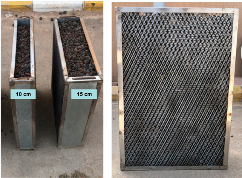
Figure 2. Volcanic stone cooling pads within the aluminum frame.
