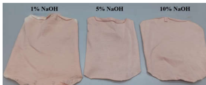
Figure 9. Cotton mesh dyed with different concentrations of NaOH (1%, 5%, 10% NaOH) after wear caused by the water fastness test.
