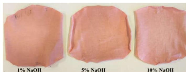
Figure 4. Cotton mesh dyed with pine cone extracts (1%, 5%, 10% NaOH).
