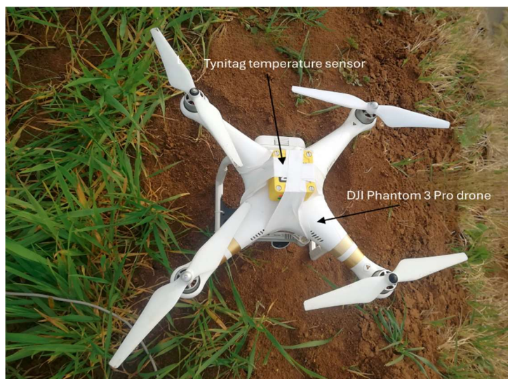
Figure 2. Tinytag sensor mounted on a drone, used in the vertical measurement of air temperature (photo by the author).
