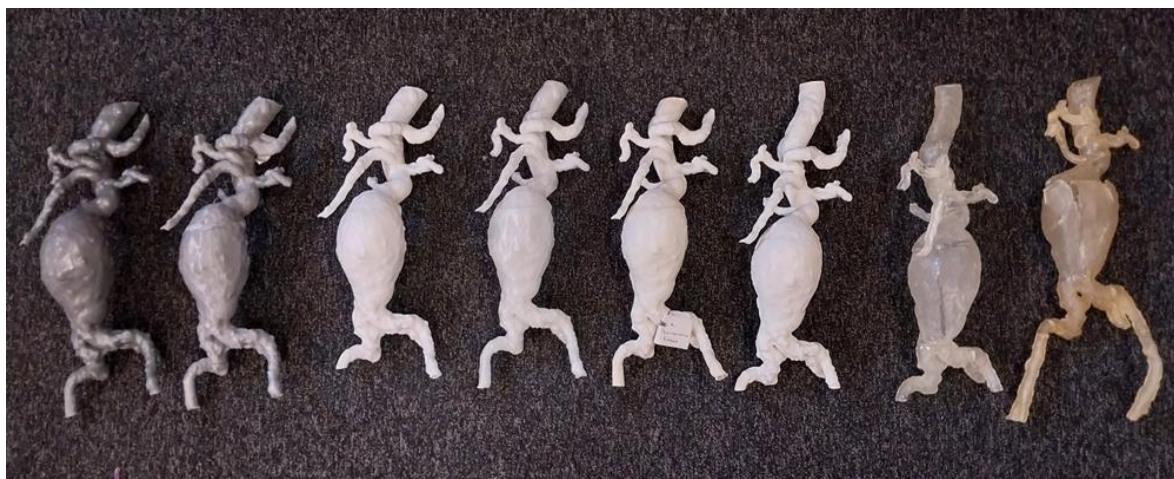
Figure 2. Variety of plastics and resins for initial material selection. From left to right: V2 resin – draft; PETG - Polyethylene Terephthalate glycol; PLA - Polylactic acid; HIPS - High Impact Polystyrene; PMMA - Polymethacrylate; TPU – Thermoplastic polyurethane; 60C resin – Tough white, TPU - Polyurethane and rubber, soft & very soft.
