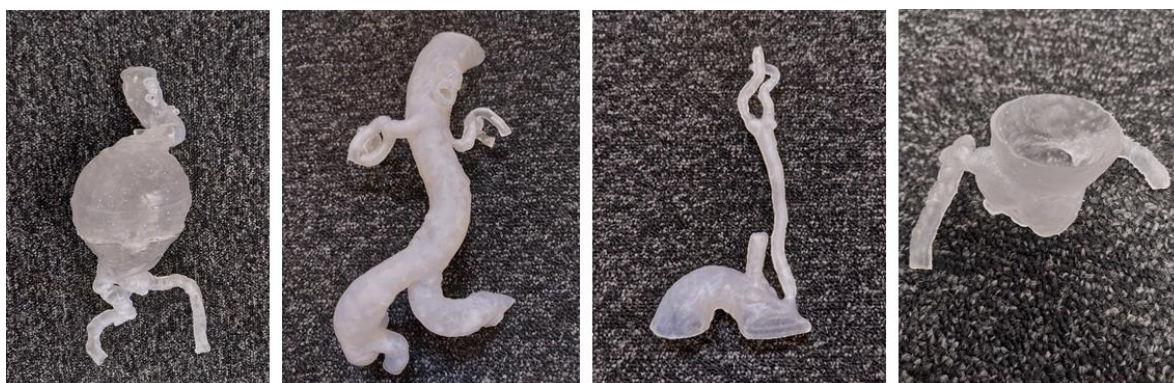
Figure 3. The four 3DPPVM printed in elastic resin (Formlabs elastic resin 50A) for clinical assessment. In order left to right: Abdominal aortic aneurysm, left renal artery stenosis, left internal carotid artery stenosis, and right coronary artery stenosis.
