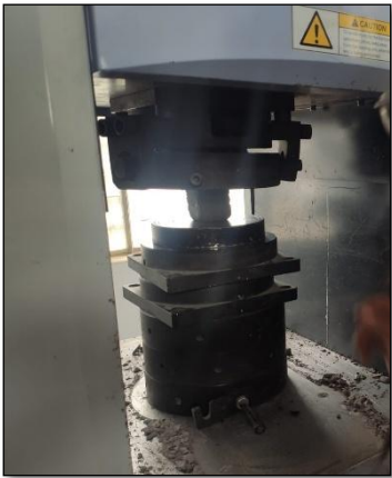
Figure 1. Compression test of 50 mm mortar cubes.
