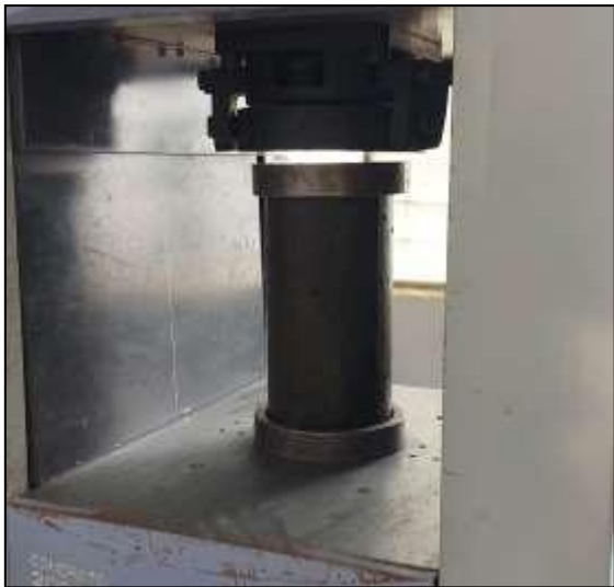
Figure 3. Compressive strength testing of cylindrical concrete samples.
