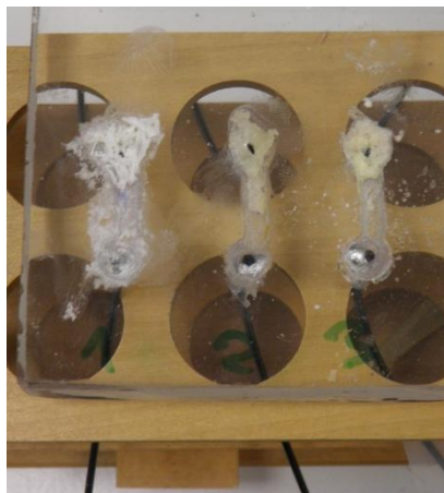
Figure 7. Three electrode pairs using liquid Ga-In alloys (bottom: bare, top: covered with chitin with an electrolyte channel in a polyacrylate support. The black lines are the conductive PLA pieces used to connect the electrodes to a voltmeter (outside of picture) without introducing additional metals. Left: pure Ga-Al, center: with “Auerstein”, right: with Al. Note the black dots in the central bare electrode (presumably magnetite). Fe level in chitin does decrease during operation, probably because of extraction by SCN - and oxidation. Final Ce levels in the central setup are some 23 times that of La.
